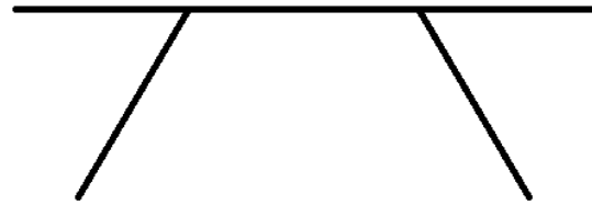
Truncated A-Frame Bridge
